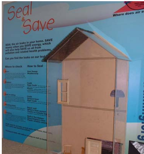
The new Seal and Save exhibit, created with a grant from the Home Depot Foundation, shows typical home air leaks. Students can seal the leaks with rope caulk.
